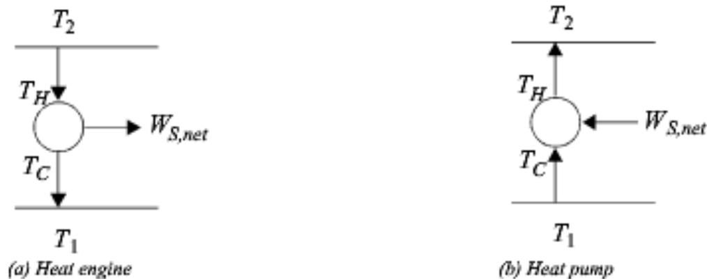
**Figure 4.5** Schematic of a heat engine (a) and heat pump (b). The temperatures of the reservoirs are not required to match the reversible engine temperatures, but work is optimized if they do, as discussed in the text.
