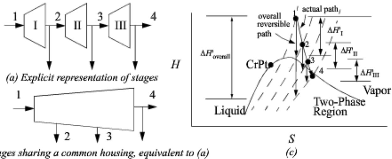
**Figure 4.11** Illustration that overall efficiency of an adiabatic turbine will be higher than the efficiency of the individual stages.
