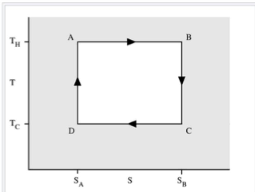
Figure 2: A Carnot cycle acting as a heat engine, illustrated on a temperature-entropy diagram. The cycle takes place between a hot reservoir at temperature  $T_H$  and a cold reservoir at temperature  $T_C$ . The vertical axis is temperature, the horizontal axis is entropy.
