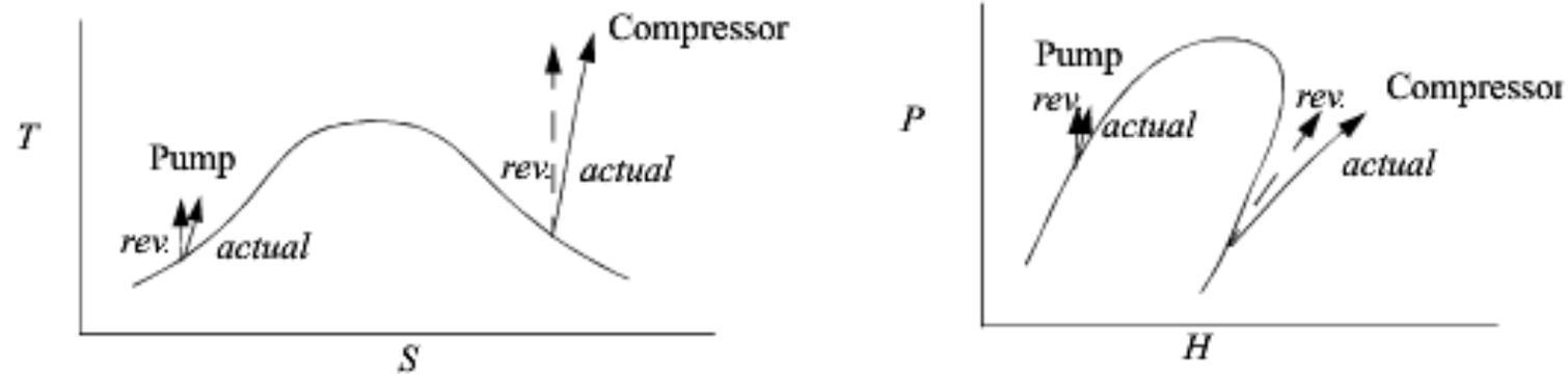
**Figure 4.12** Illustrations of pathways for reversible and irreversible pumps and compressors. The  $P$ - $H$  diagram is for a system like Fig. 4.7(a).
