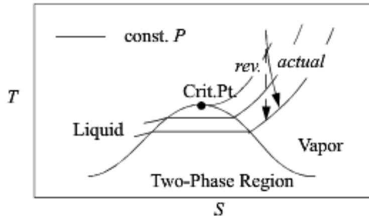
**Figure 4.9** Illustration of a reversible and actual (irreversible) turbine on a T-S diagram.
