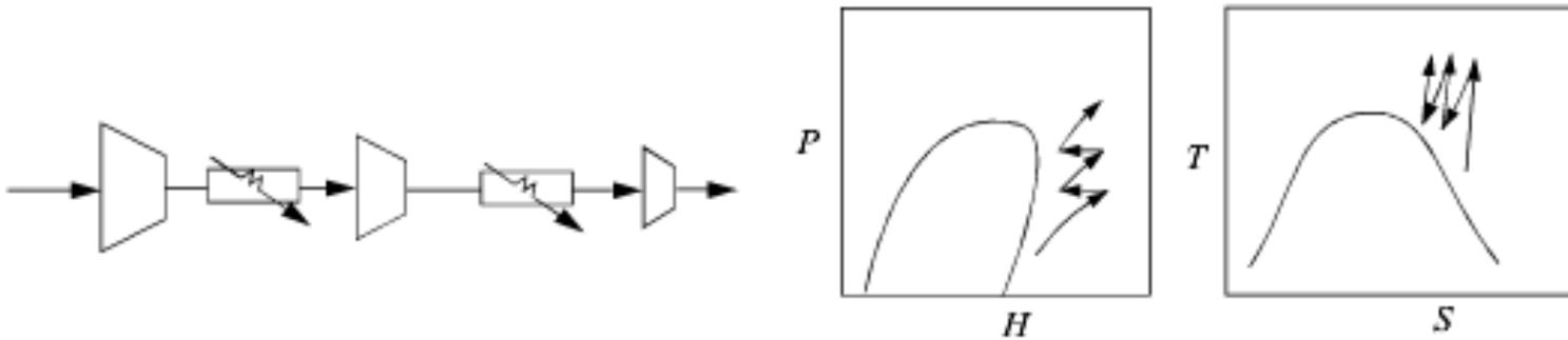
**Figure 4.13** Illustration of a multistage compression and the corresponding  $P$ - $H$  diagram. On the  $P$ - $H$  diagram, the compressors appear as the curves of increasing pressure and the heat exchangers are the horizontal lines at constant pressure.
